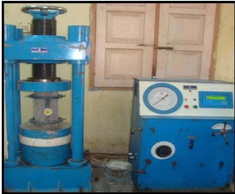
Fig: 4 Test on Concrete Cylinders for E for concrete
