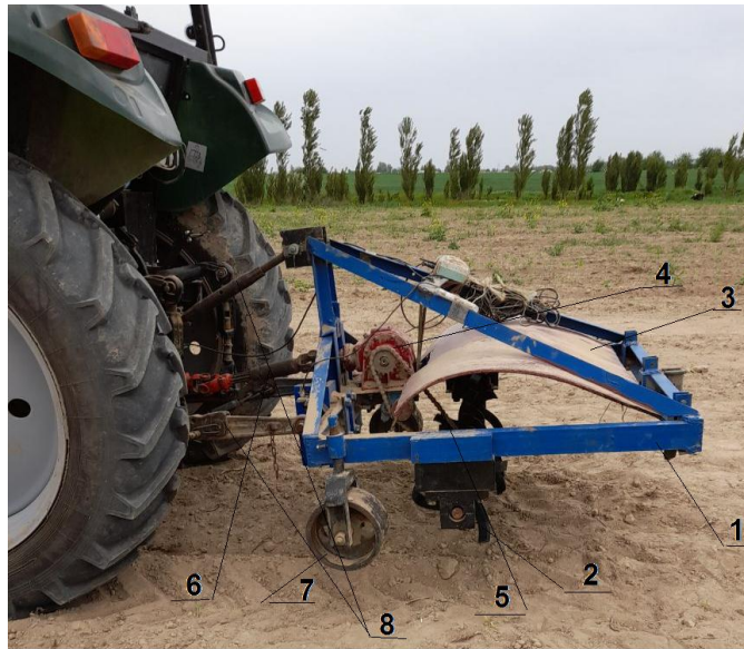
1-rama; 2 rotary softeners; 3- protective barrier to prevent the scattering of crushed soil; 4 rotary softener motion transmission device; 5.6-motion transmitter; 7 base wheels; 8 -device of the device on the tractor.
