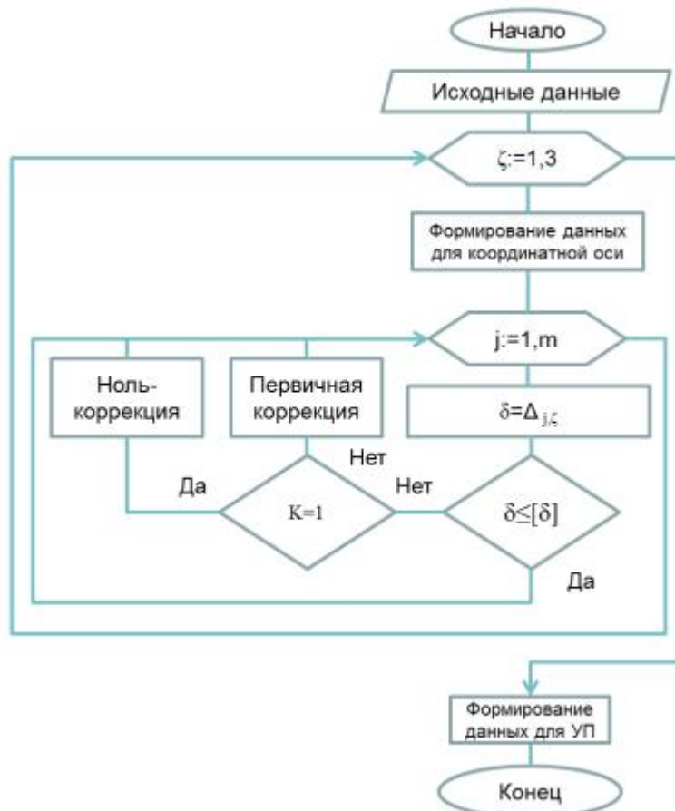
Figure 4-Algorithm for applying "zero-correction" and "primary correction"
